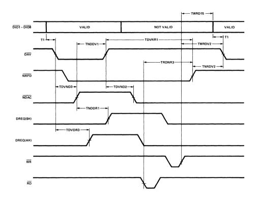
Figure C-1. 3-Wire Handshake Timing at 8291.
